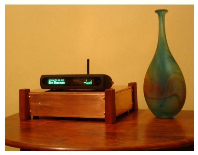
This is a high-performance audio power amplifier using the LM3886. Its home is to bi-amp my Linn Keosa floorstanding loudspeakers (using their passive crossover, but separate amplifier channels for top and mid/bass) with <u>SqueezeBox2</u> as source. There's no preamp; volume control is digital, internal to the SB2. The high output impedance means this amplifier should work really well with single-driver full-range speakers too.
